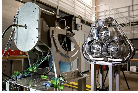
Figure 2. Photograph of the current solar simulator and receiver test setup
