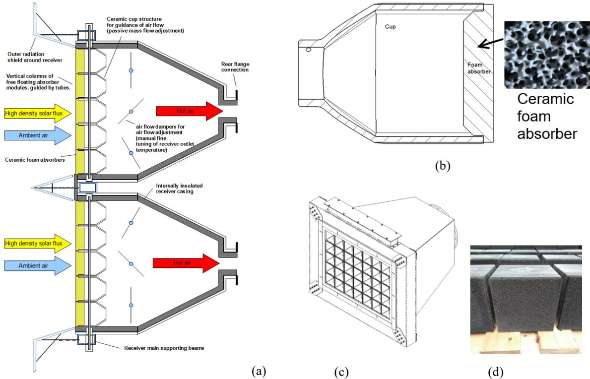
Fig. 1: Open Volumetric Air Receiver (OVAR) concept (a); Stackable absorber module (b); CAPTURE  $300\text{ kW}_{\text{th}}$  prototype without foam absorbers (c); CAPTURE absorber modules before receiver mounting (d).
